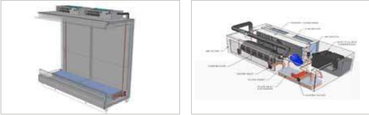
Diagram of Carter display case (left) with positioning and construction of condensing unit (right)
